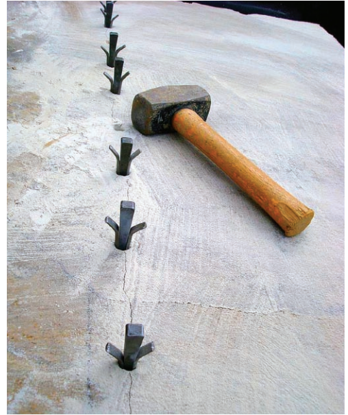
Photo 2. Modern example of 'drill and feather' method. (Photo courtesy of Anna Frodesiak)
